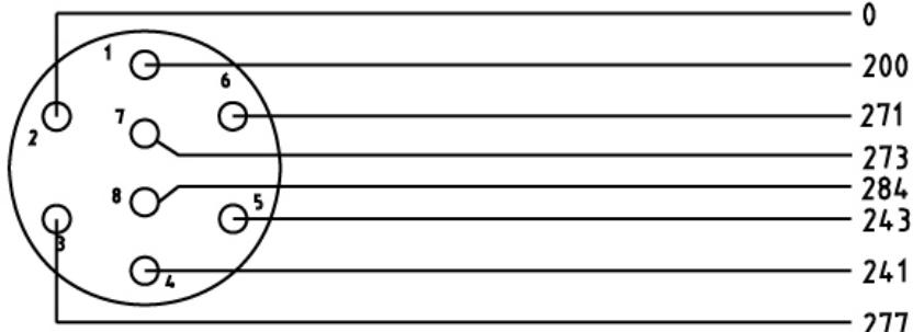
Wiring definition of 8-core aviation plug(socket):
