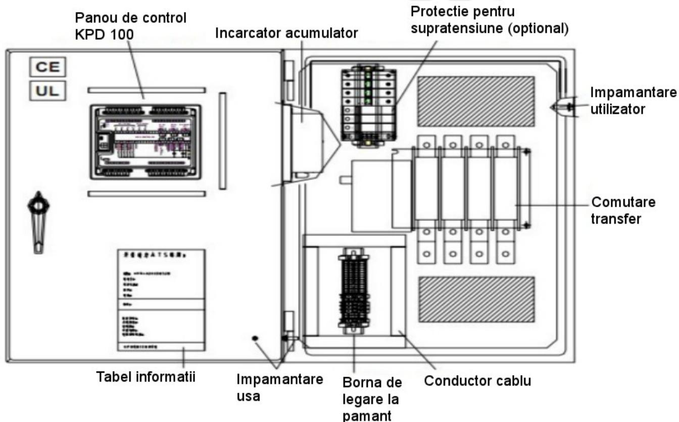
**Fig.3-1 Cutie ATS seria KPA: 200A, comutator transfer cu 4-poli**
